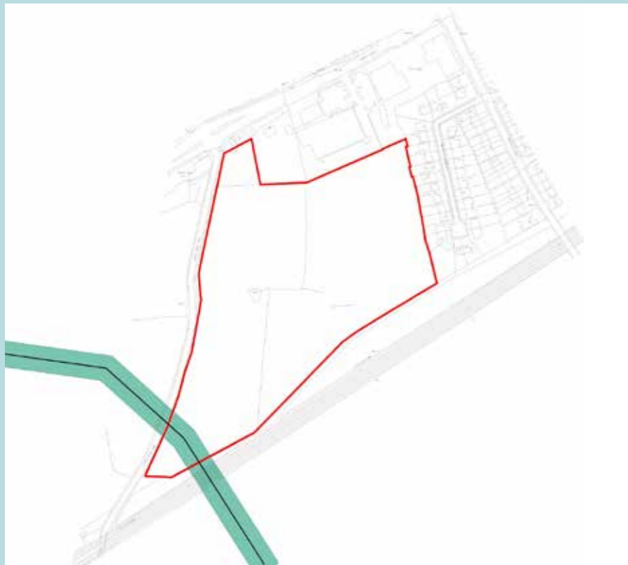
Site Location Plan with high pressure gas main and 28m corridor highlighted.
