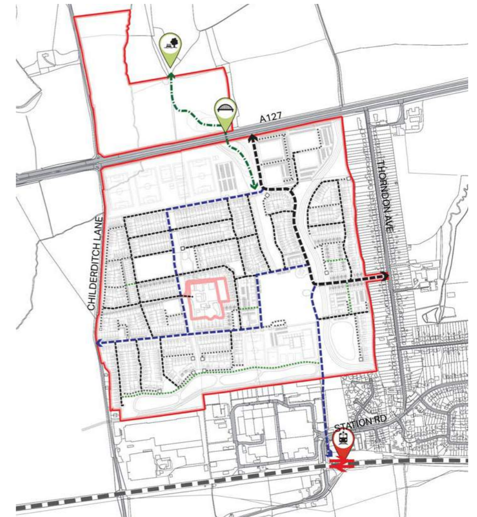
Fig 3.13 - Secondary road network
