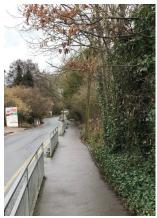
The footway along the frontage of St Helen's school suffers from poor alignment and inconsistent width. The guard railing and wooden edging within this area significantly limits the available footway width and presents the potential for obstructions and trip hazards along the link (left).
