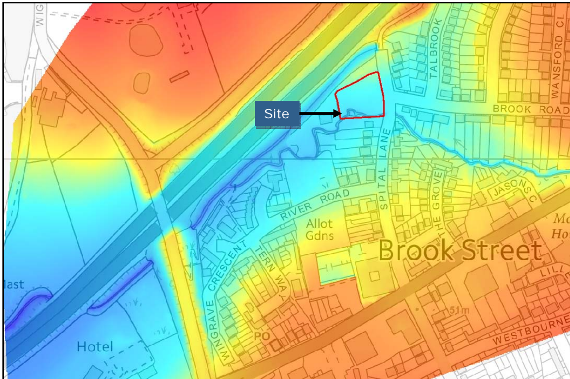
Figure 2: Ground level variation across the study area and OS map using LIDAR data (Source: Promap 2015)
