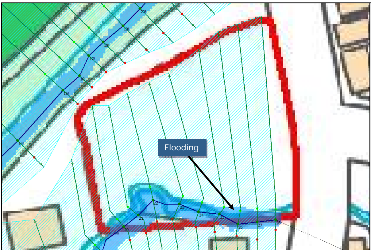
Figure 29: Plan view of the flood extent during a climate change 1 in 20 year event
